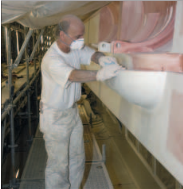
Left —Surface coloring is particularly important to this member of the crew—the detail sander. Note that he is working only on the radiused panels, sharp edges, and inside corners in the life-raft-canister storage section of the bulwarks. The flat-panel sections ahead and aft of this spot are left to someone else. Above, right —Coloring the matte finish of each but the last top-coat layer's surface allows the sanding crew to spot high and low areas and confirm 100% sanding coverage of each area. Sanding strokes are on the diagonal, lower right to upper left, followed by a similar number from upper right to lower left. Above —Because both coarse and fine fairing materials are applied with a blade, critical edge details such as the overhang shown here will need only minor sanding.
