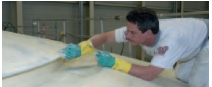
Left —Surface coloring is particularly important to this member of the crew—the detail sander. Note that he is working only on the radiused panels, sharp edges, and inside corners in the life-raft-canister storage section of the bulwarks. The flat-panel sections ahead and aft of this spot are left to someone else. Above, right —Coloring the matte finish of each but the last top-coat layer's surface allows the sanding crew to spot high and low areas and confirm 100% sanding coverage of each area. Sanding strokes are on the diagonal, lower right to upper left, followed by a similar number from upper right to lower left. Above —Because both coarse and fine fairing materials are applied with a blade, critical edge details such as the overhang shown here will need only minor sanding.
