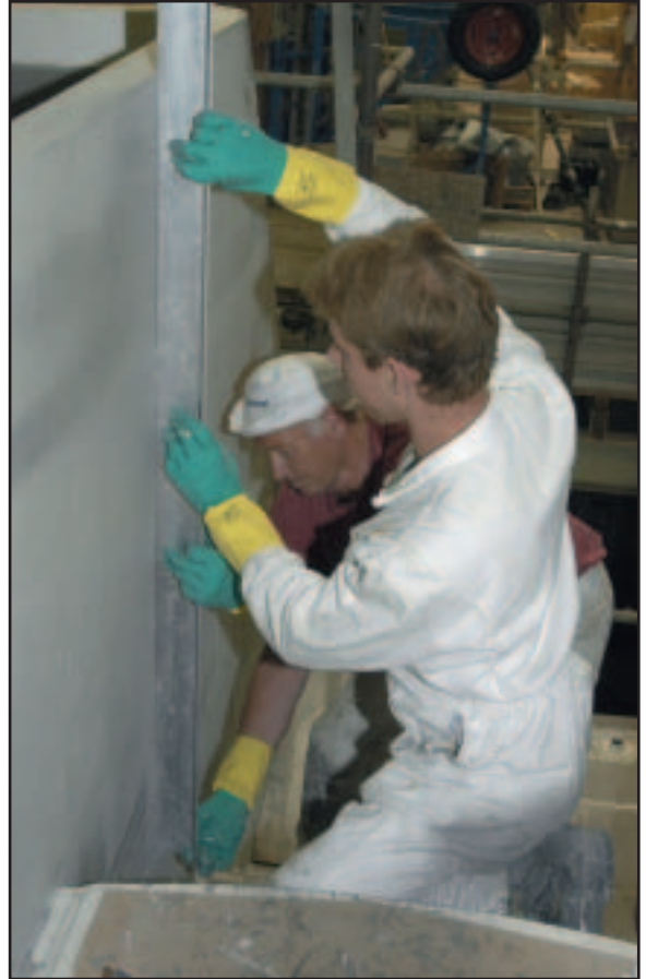
Facing page —The reflections on these complex curves and inside and outside corners show no jagged edges—a sign of a high-quality fairing job underneath carefully sanded primer and topcoat layers. Above —This equipment foundation receives the same methodical fairing, priming, sanding, and topcoating steps as a hull’s panels and topsides. Right —Sighting underneath an aluminum straightedge during a “dry run”—that is, without putty—allows the fairing crew to spot high and low locations before they apply any more material. Notice the matte and shiny surface bands left behind by a brief longboarding that takes down only the high spots. The efficient time to sand off the high spots is at the gray fairing stage, shown here.
