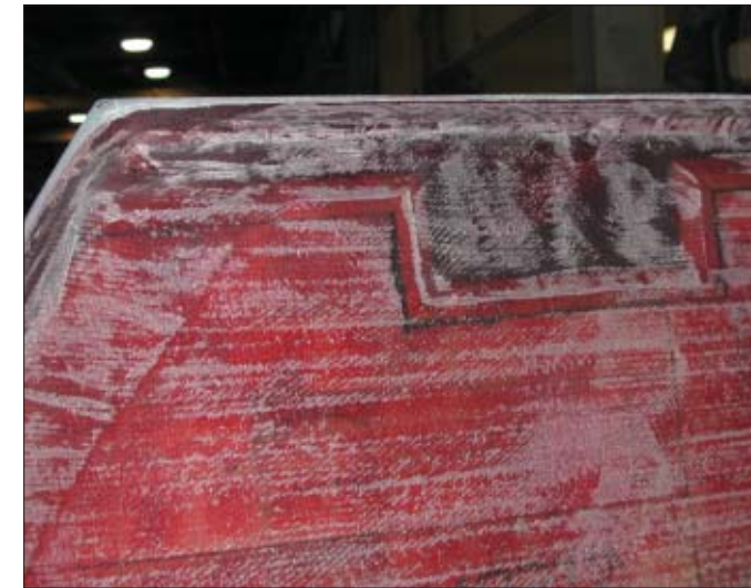
Left —Note the mitered inside and outside corners on the tapered edge strips, and the complete kerf fill in the core of this infused hull. Right —Woven and knit reinforcements don't register well against square core edges, especially on thick cores. Chopped-strand mat, whether from a roll or a choppergun, is not much more effective.
