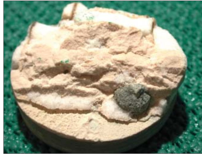
Left —In this sample, the core was not primed before being placed on an adhesive layer that was too thin. Incomplete bondline contact produced large air pockets that printed through the thin, dark-colored exterior skin. Right —Coarse aggregates belong in concrete, not core-bonding putty. In other coupons from the same boat, aggregate prevented the core from registering against the skin.
