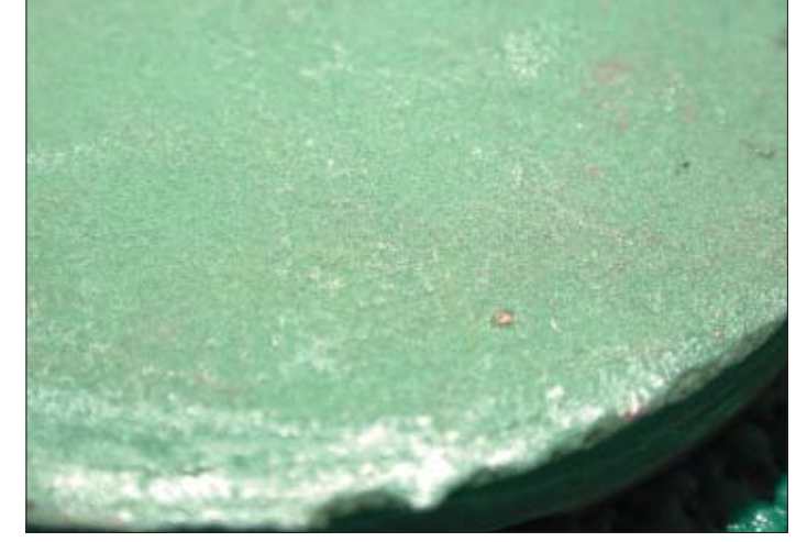
Left —Uncompressed trowel grooves in the core-bedding putty characterize a classic neverbond. Right —This unusual example shows a "kissing" neverbond: the putty was still soft enough to pick up the cellular texture of the core, but was starting to gel, and unable to establish a bond. Note the pink priming resin on the lower part of the coupon. The absence of core material attached to the priming resin indicates that it had not gelled—when the putty already had.
