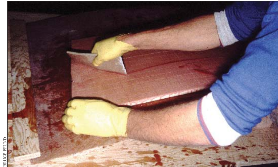
A thin piece of plywood bowed between two wooden cleats makes a simple core-kerf-wetout fixture. Placing a dogleg overhang at the fixture's opposite side secures the loose end of the sheet for bending.
