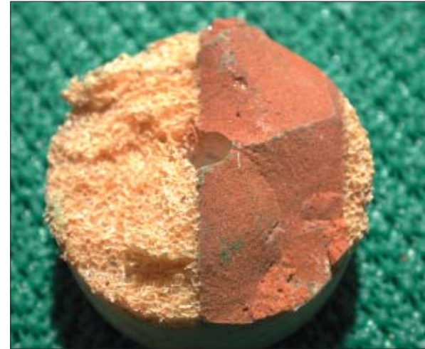
Left —The void shown here caused a linear band of print-through on the exterior of a black-gelcoated topsides panel. A putty bevel might have printed, too. A tapered foam edge strip, from the same density foam, would transition the panel's thermal properties more gradually. Right —When the adhesive thickness in the butt joints between core panels approaches or exceeds the thickness of the core, it is probably too thick. For putty filling, butt seams 50% narrower (or less) than the core thickness are preferable. For infusion, tight fits are better—provided resin flow paths are not smaller or more restricted than elsewhere in the core's flow channels.
