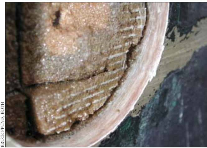
Left —This foam core was installed scrim-out into a wet-chop bonding layer. The chop, though, was not wet enough to dissolve the scrim's styrene-soluble hot-melt adhesive network on the core surface. The kerfs in the coupons removed had no visible resin in them, indicating that the bondline face of the core was probably never effectively primed with resin. Right —The core block failures were completely within the core—the preferred failure mode—except where the core was not in contact with the wet-chop bedding layer.
