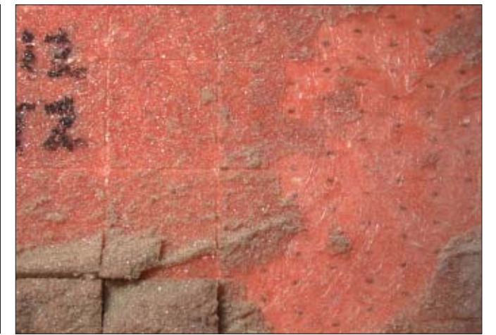
Left —This foam core was installed scrim-out into a wet-chop bonding layer. The chop, though, was not wet enough to dissolve the scrim's styrene-soluble hot-melt adhesive network on the core surface. The kerfs in the coupons removed had no visible resin in them, indicating that the bondline face of the core was probably never effectively primed with resin. Right —The core block failures were completely within the core—the preferred failure mode—except where the core was not in contact with the wet-chop bedding layer.
