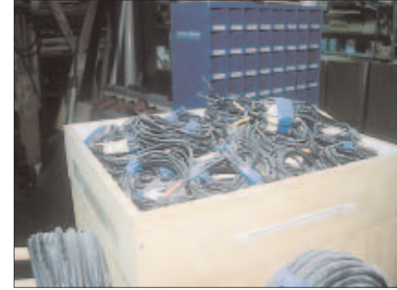
Left —The Goetz shop has a substantial inventory of neatly organized thermocouples with standard lengths of wiring and plug terminations, all kept in a box on top of a roll-around storage stand. Right —Six individual thermocouple cables plug into these junction boxes; the larger multi-connector "jumbo cable" is run back to the interface box. This way, it's easier to keep the channels organized, and there is less cable lying on the shop floor, where it could be damaged.
